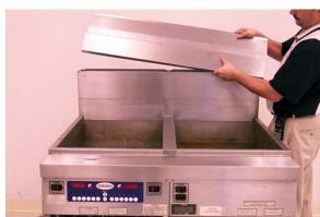
Removing the flue cap.
